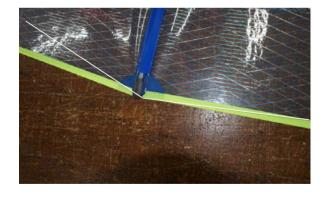
If fully battened, the battens shall be in the sail and tensioned until the batten pocket is smooth
